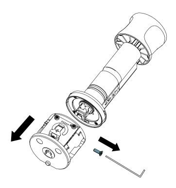
5. Loosen the back-plate screw with a Torx T6 tool.
