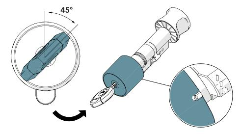
2. Use a Torx T6 tool to loosen the fixing screw by rotating it clockwise (left-hand thread).
