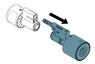
3. Slide the shaft into the lock unit and make sure that the seal is in the correct place. Secure the extension assembly with the provided screw. Use a Torx T10 tool (tightening torque 2.5 Nm).
