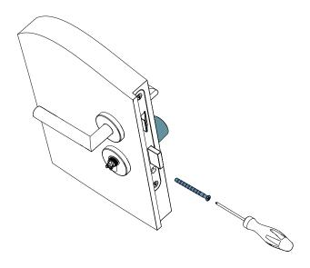
4. Install the electronic knob as described in chapter "6. Removing and installing the electric knob".
