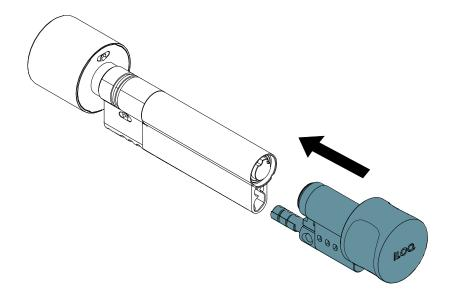
6. Secure the lock unit with the three fixing screws set aside earlier. Use a tightening torque of 0.55 ... 0.65 Nm.
