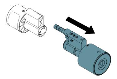
3. Slide the shaft into the lock unit and make sure that the seal is in the correct place. Secure the extension assembly with the provided screw. Use a Torx T10 tool (tightening torque 2.5 Nm). Make sure that the black O-ring is between the extension assembly and the lock unit. Make sure that the housing is aligned correctly.
