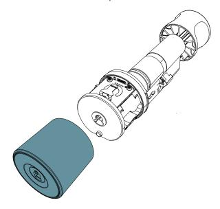
4. Remove the side screw counterclockwise with a Torx T6 tool and carefully detach the knob with the PCB.
