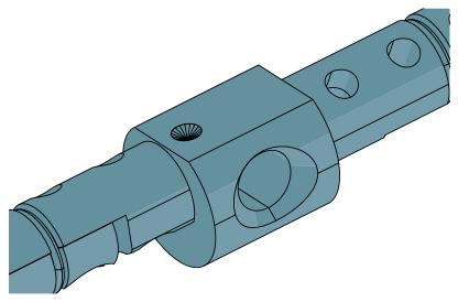
If the long-neck version is used in a door with the complete DIN cut-out, to improve the pulling protection safety of the cylinder, change the long-neck backbone to the DIN backbone (A5.009). The long neck backbone is slightly shorter than the DIN backbone. Or, it is also possible to rotate the existing backbone (outside to inside).
