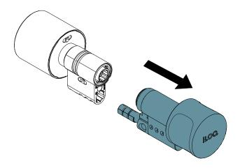
3. Put the shaft into lock unit and check that the seal is in the correct place. Secure the extension assembly with the provided screw.
