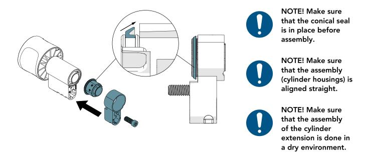
4. Slide the assembly with the backbone into the assembly with the extension piece and align the housings.
