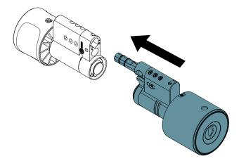
5. Secure the lock unit with the three body fixing screws set aside earlier. Use a tightening torque of 0.55 ... 0.65 Nm.
