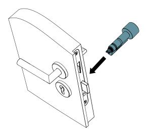
3. Secure the cylinder to the lock case with an iLOQ fixing screw (A10.64, part of the delivery). Use a tightening torque of  $0.9 \dots 1.1 \text{ Nm}$ . If necessary, cut the screw to the correct length (calculation screw length: L = backset + 10 mm).
