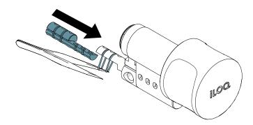
6. Slide the assembly with the backbone into the assembly with the extension piece and align the housings.
