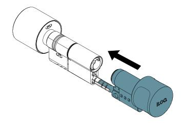
7. Secure the lock unit with the body fixing screws. Use a tightening torque of 0.55 ... 0.65 Nm.
