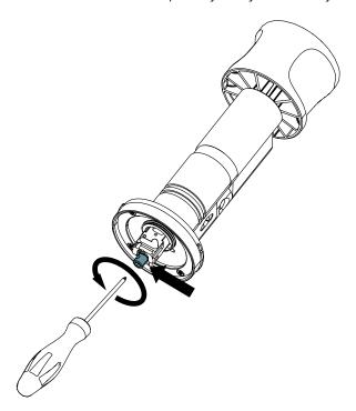
6. Rotate the backplate counterclockwise and pull it off.
