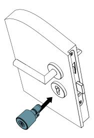
2. Secure the cylinder to the lock case with an iLOQ fixing screw (A10.64, part of the delivery). Use a tightening torque of 0.9...1.1 Nm. If necessary, cut the screw to the correct length (calculation screw length: L = backset + 10 mm).
