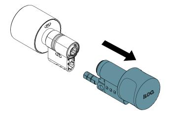
3. Put the shaft into lock unit and check that the seal is in the correct place. Secure the extension assembly with the provided screw. Use a Torx T10 tool (tightening torque 2.5 Nm).
