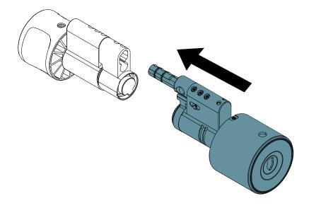
6. Secure the lock unit with the three body fixing screws set aside earlier. Use a tightening torque of  $0.55\ldots0.65\,\mathrm{Nm}$ .
