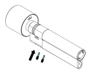
5. Slide the assembly with the backbone into the assembly with the extension piece and align the housings.
