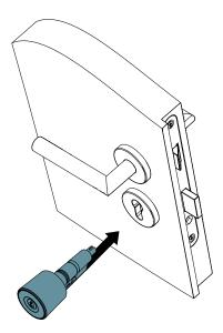
3. Secure the cylinder to the lock case with an iLOQ fixing screw (A10.64, part of the delivery). Use a tightening torque of 0.9...1.1 Nm. If necessary, cut the screw to the correct length (calculation screw length: L = backset + 10 mm).
