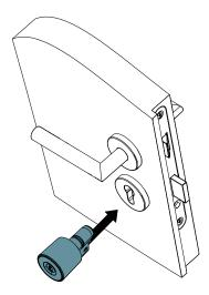
2. Secure the cylinder to the lock case with an iLOQ fixing screw (A10.64, part of the delivery). Use a tightening torque of 0.9...1.1 Nm. If necessary, cut the screw to the correct length (calculation screw length: L = backset + 10 mm).
