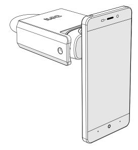
1. Present a valid key to the reader knob to activate the lock. Wait until the key shows a green light to indicate that the lock is unlocked.
