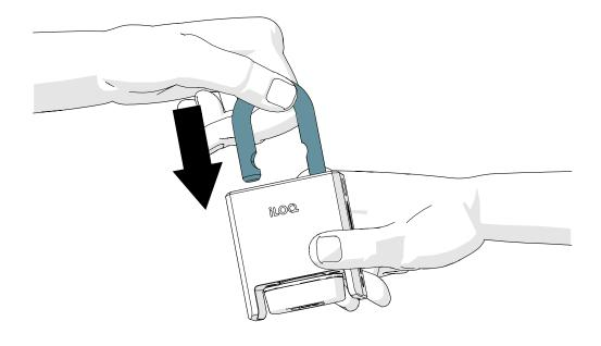
2. Present a valid key to the reader knob to activate the lock. Wait until the key shows a green light to indicate that the lock is unlocked.
