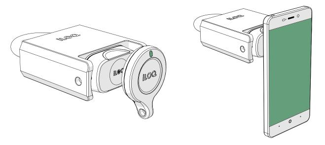
3. Turn the reader knob 180° counterclockwise. The lock stays in the open-status for 5 to 15 seconds and automatically returns back to the locked-status if not opened (depending on the configured lock opening time).
