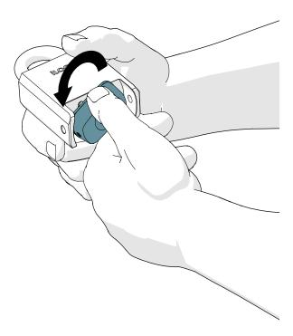
4. After closing the lock, ensure that the knob is in locked position and the padlock remains closed.
