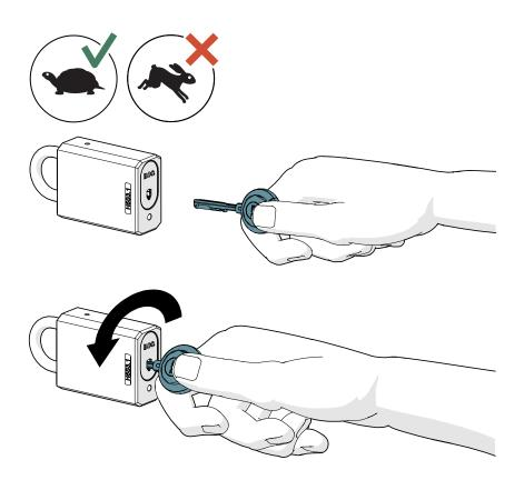
3. After closing the lock, ensure that the knob is in locked position and the padlock remains closed.
