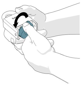
3. After closing the lock, ensure that the knob is in locked position and the padlock remains closed.
