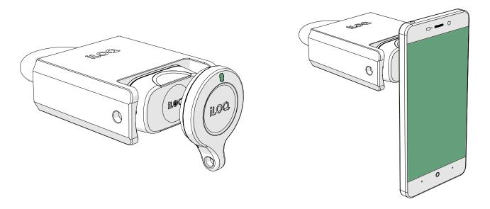
2. Turn the reader knob clockwise 180°. The lock stays in the open-status for 5 to 15 seconds and automatically returns back to the locked-status if not opened (depending on the configured lock opening time).
