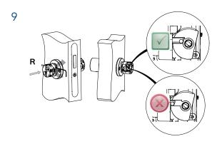
**R.** Put the knob on its place and slide the FFC out from the knob slot. Tighten the knob screw with TORX 6 tool.
