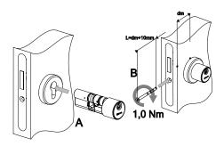
**A.** Slide lock cylinder through the lock case.
