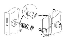
**P.** Slide lock cylinder through the lock case. Take care that FFC doesn't get damaged.
