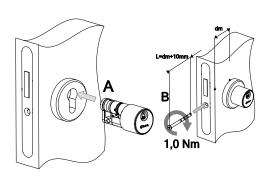
A. Slide lock cylinder through the lock case.
