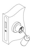
After 10 000 usages, clean contact rolls lightly with lint-free cotton pad. Spray small amount of high quality lock oil i.e. CRC lock oil (with PTFE) onto contact rolls.
