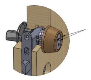
Align cylinder and escutcheon surfaces. Use cylinder extension piece, if needed.
