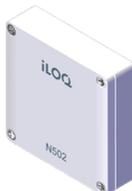
The Door Module is connected to a Net Bridge via RS485 bus wiring. The location of the Door Module should be in close proximity to the door. The maximum cable length from the Door Module to a lock cylinder or RFID reader is 10m. The Door Module contains two relays with individual functions that can be edited in the iLOQ Manager. At the connected door / magnet contact, the door status is obtained as open / closed.
