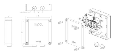
The iLOQ N501 4G Standalone Door Module is a device located in the vicinity of a door, and it controls devices installed on the door, such as a lock cylinder, an iLOQ Online Reader, an electric lock, an electric strike plate, a magnet lock, and so on. The iLOQ N501 4G Door Module is equipped with a pre-installed 4G connection to the iLOQ Cloud. With the iLOQ N501 4G Door Module, the remote or otherwise hard-to-wire door environments can be easily connected to be a part of the iLOQ Online system.
