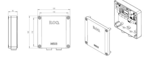
The iLOQ N503 Offline Door Module is located in the vicinity of a door, and it controls devices installed on the door, such as iLOQ NFC Reader, an electric lock, an electric strike plate, a magnet lock, and so on. N503 has several different use cases, and it can be used both as unprogrammed in combination with connected C5 cylinders or programmed as a Lock with the connected iLOQ NFC Readers.
