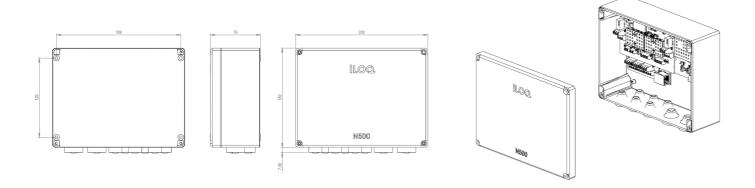
The iLOQ N507 Online I/O Module is a bus device located in the vicinity of a door, and it controls devices installed on the door, such as an electric lock, an electric strike plate, a magnet lock, and so on. The N507 Online I/O Module is hosted by a Net Bridge or another N507; it does not operate independently. The N507 Online I/O Module has several different use cases, and it can be used both as unprogrammed or programmed.
