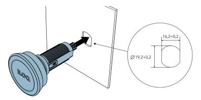
2. Install and tighten the cylinder fixing nut to a torque of 8 Nm.
