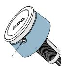
2. Insert the lock cylinder body through the hole in the door.
