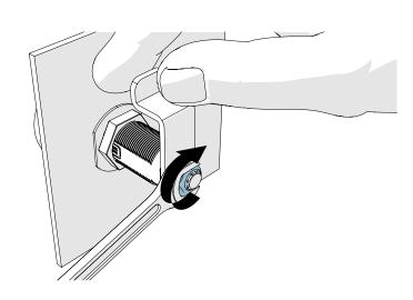
4. Use the locking washer to secure the latch fixing nut once tightened.
