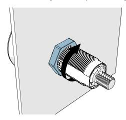
3. Install the latch, locking washer and latch fixing nut (1 Nm torque).
