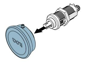
3. Slide the new reader knob onto the neck so that the screw hole is facing the same direction as the two knob adjustment slots in the neck.
