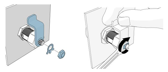
5. Use the locking washer to secure the latch fixing nut once tightened.
