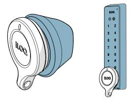
2. Wait until the K55S.1 Key Fob shows a green light to indicate that the cylinder is unlocked. The K55S.1 Key Fob shows an amber light while communicating.
