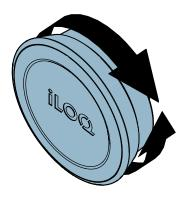
NOTE! Depending on the configuration, the lock will stay in the open status for 5-15 seconds. Do not force the knob.
