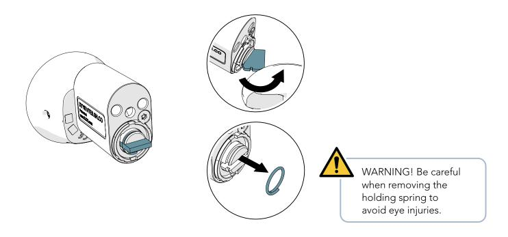
2. Turn the tail-plugin fixing T10 screw carefully to the left and remove the fixing screw.
