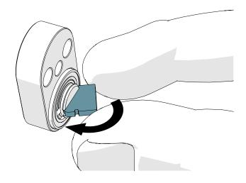
3. Install the cylinder centering piece between the lock case and the lock cylinder.
