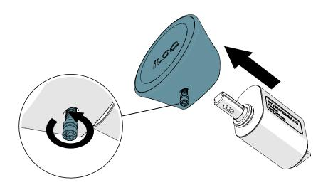
2. Adjust the knob to the right distance and tighten the screw. Use a tightening torque of 1.5 Nm.
