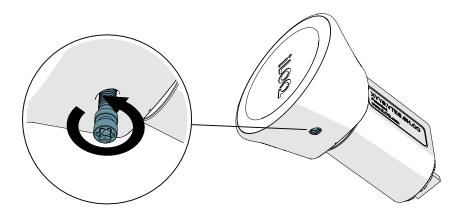
2. Adjust the knob to the right distance and tighten the screw. Use a tightening torque of 1.5 Nm.
