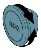
NOTE! After 5 seconds (default), the cylinder will automatically be locked. When the cylinder is locked, the iLOQ Reader Knob cannot be rotated.
