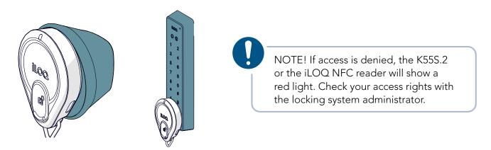
3. Wait until the K55S.2 shows a green light to indicate that access is granted. The K55S.2 shows an amber light while scanning the iLOQ NFC reader and shows a purple light when communicating with the iLOQ NFC reader.
