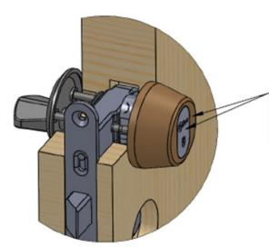
Align cylinder and escutcheon surfaces. Use cylinder position extension piece, if needed.
