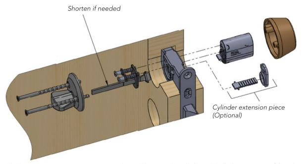
A cylinder extension piece iLOQ A10.33 must be used between the cylinder and the lock case in case of the cylinder height adjustment is necessary. When using the extension piece, also use appropriate longer tail piece. The extension piece must be used also if there is a pin or similar protruding from the lock case surface and can push oneself on the cylinder rear body.
