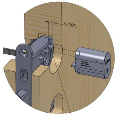
IMPORTANT! Screw length must not exceed 6 mm, too long screw will damage lock cylinder.
